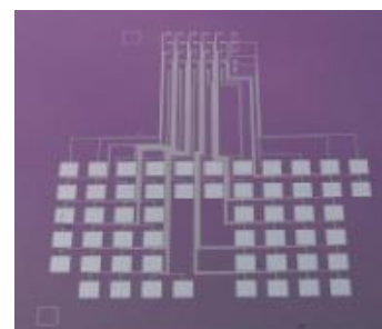
Array of 30 micro-SOFC integrated on Si wafer
