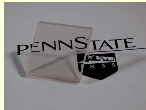
Stacked Er:YAG composite (tape cast), 25 x 25 x 3 mm (0/0.25/0.50% Er:YAG – bottom to top)
