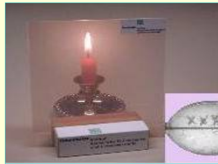
Transparent components of sintered corundum with sub- \mu m microstructure
