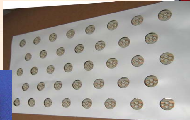
Arrangement of R-G-B pixels on metal plate with reflector
