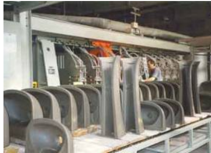
Pressure slip casting
