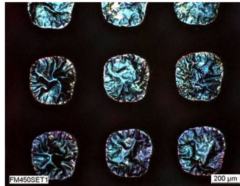
membrane after heat treatment at 450 °C
