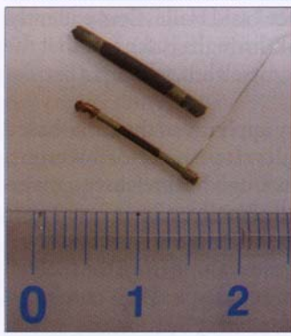
Cellular science: researchers at AIST in Japan believe that the tubular SOFC design has a number of advantages over planar architectures. Left: two AIST micro SOFCs, one measuring 1.6 mm in diameter and the other 0.8 mm. Right: close-up of the end of a micro SOFC tube showing the cathode (outside)/electrolyte/anode trilayer.
